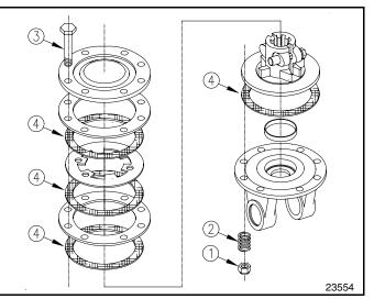
Clutch Disassembly Figure 5-3
